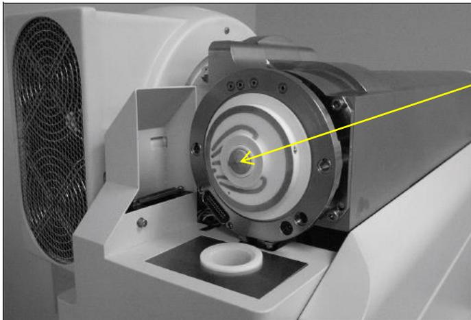
**Orifice** (with ion source and orifice cover removed)
