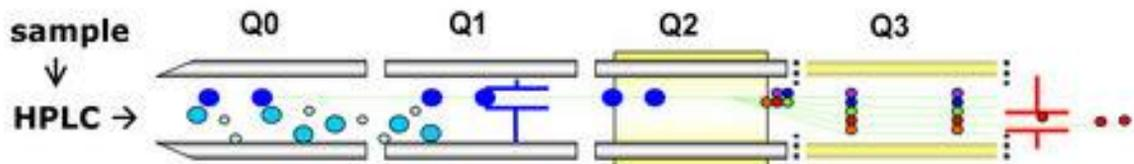
The succinate ions (shown in blue) will be filtered away from other ions in Q1, accelerate into the collision gas and undergo fragmentation in Q2. All of the fragment ions will escape the collision cell (Q2) and enter Q3. In Q3, the fragment ions will be scanned for mass determination.
