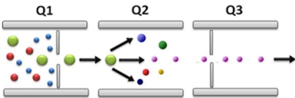
The higher the collision energy, the greater the fragmentation. If the CE is too low, the molecule undergoes inefficient fragmentation. Raising the CE too high can cause too much fragmentation. A CE set too high or low can drastically reduce the sensitivity of an MRM method.
