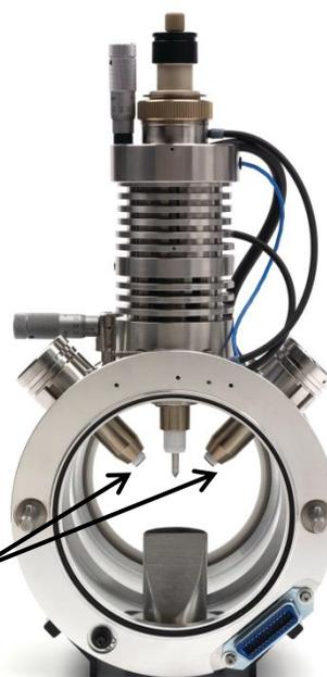
Gas 2 (**GS2**) blows out of the ceramic heaters and helps to evaporate the spray droplets.
